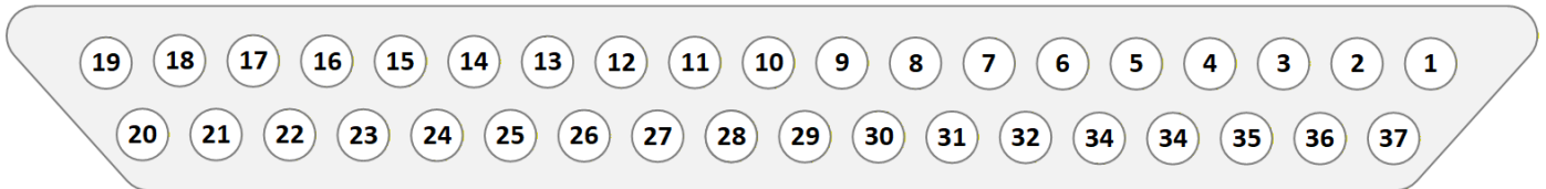
Control connector (female connector strip) on the rear of the test device (view of the test device from behind)
