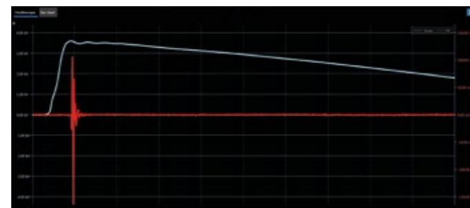
Surge voltage pulse with 150 ns rise time and PD effects
