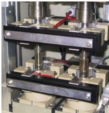
Dual station with expanding mandrel and forming tool
