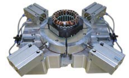
Forming tool consisting of four segments, closed condition
