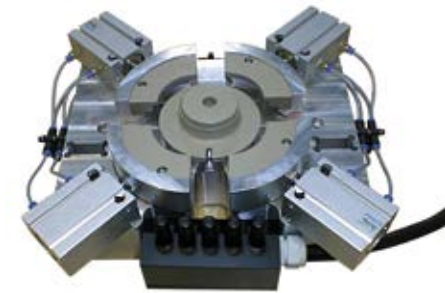
Forming tool consisting of four segments and contacting unit
