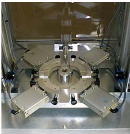
Forming tool in the bonding station
