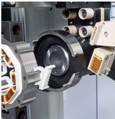
Automatic contacting unit with forming tool
