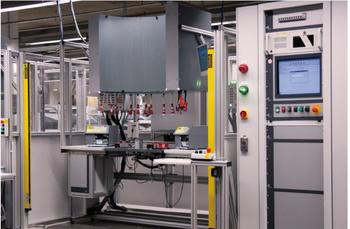
Luminaire-test system with cabin with three closed sides.
