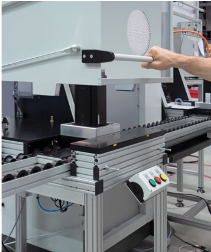
Test cover with manual roller conveyor.
